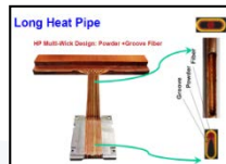
Two CPU solution : Total 1000W Heat pipe length > 600mm
